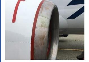
Av-DEC SpraySeal<sup>®</sup>, SF2470, is a twocomponent polyurea material engineered to create a watertight, flexible seal to protect against corrosion. Upon application, SpraySeal will protect surfaces vulnerable to Uniform Etch Corrosion.
